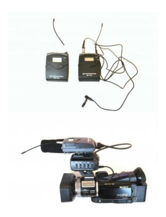
Transmitter, receiver and microphone (left) and receiver attached to the camera
