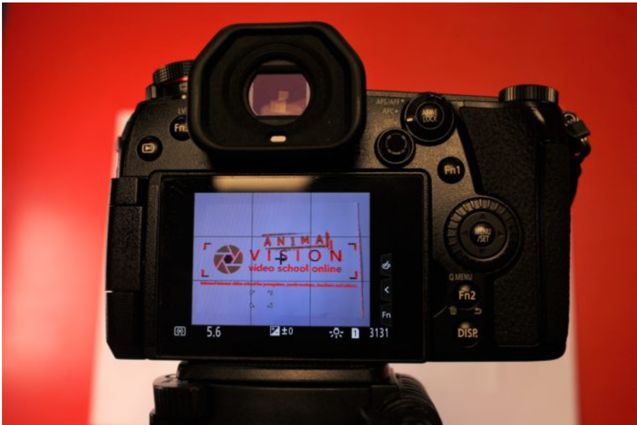
Camera Display with Peaking function (red dots)
